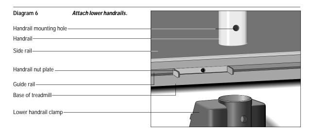
10. To mount the lower portion of the handrails, take the lower handrail clamps (J), two of the internal star washers (E), and lower handrail clamp bolts (C) out of the hardware kit. Refer to Diagram 6 while taking the following steps:
